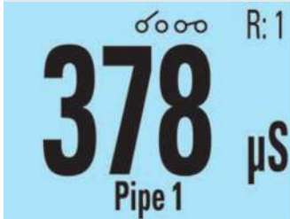
Conductivity value with measuring point (TAG)
