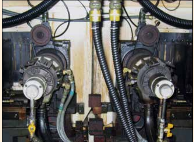
DEUBLIN 2-passge Unions on CNC Turning Center
